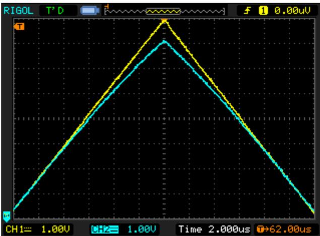
As you can see, there is no discernable difference so it can be used to replace the original Atari VDR.
