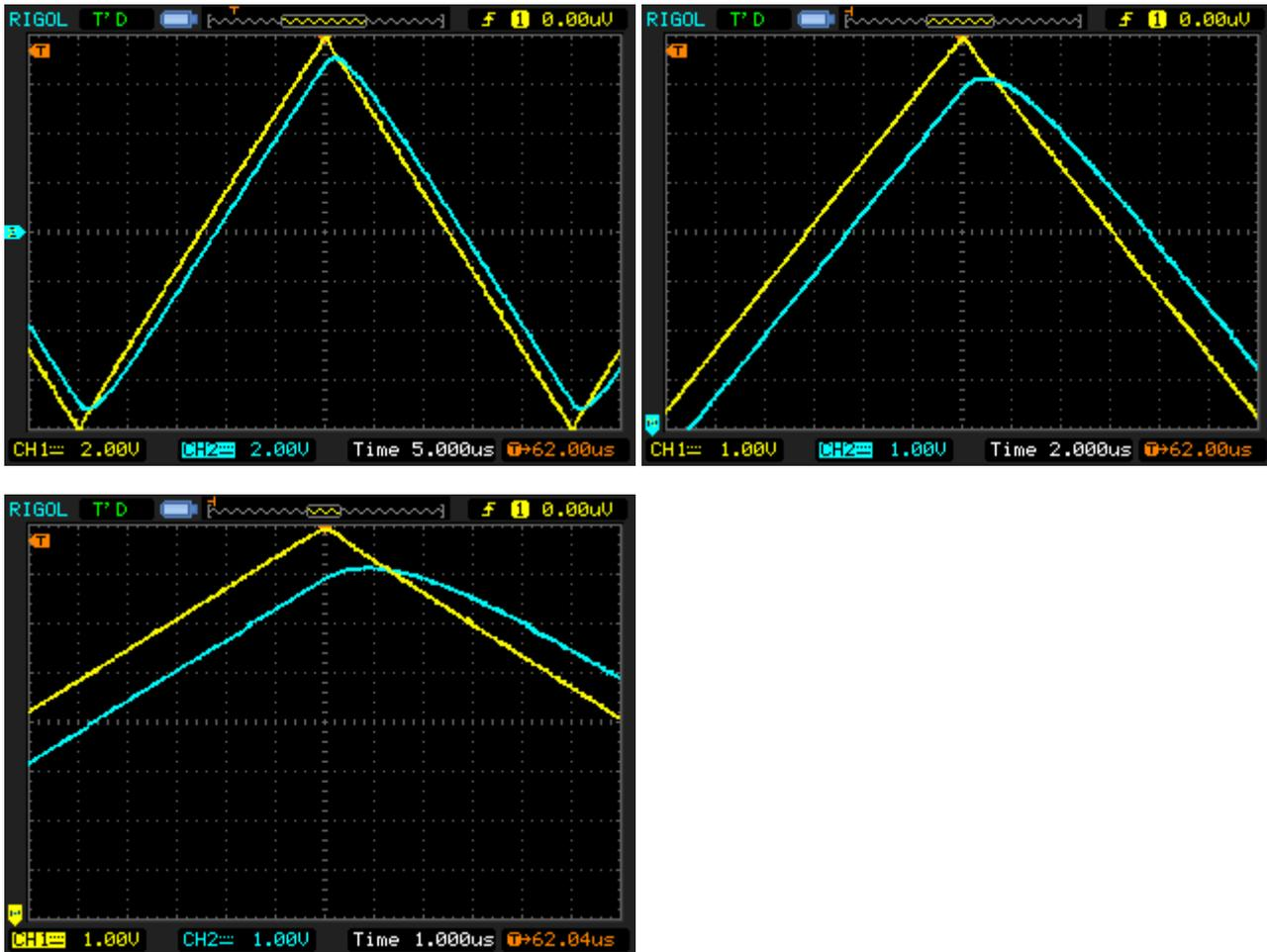
With the same input signal as used with the original VDR and the BXVDR, the blue line clearly does not follow an exponential path. Worse, a large phase shift is produced. There is simply no way then that the MOV presented here can apply the correct exponential function to the vector being drawn and therefore it cannot draw a straight diagonal vector across the CRT screen. Also, this indicates that the absolute position and length of horizontal and vertical vectors will not be accurate.
