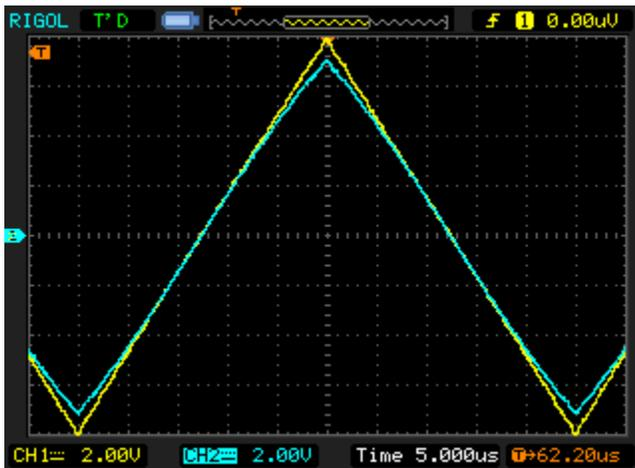
The yellow line is the input waveform, a perfect linear triangle wave. The 20 kHz signal of amplitude of +/- 8V peak is applied to the voltage divider. The blue line is the output response and it should be the same in both polarities which you can see that it is.
